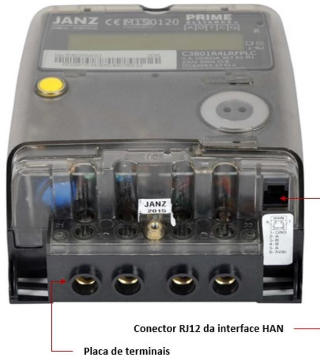
Figura 3 – ECCE monofásico PLC PRIME | JANZ C3801R4LRFPLC – vista inferior
